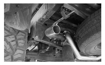
**14.** Slip a clamp (11) over the left tailpipe (7). Install its hanger rod in the rubber isolator, then slip it over the over-axle pipe. Verify 3" of insertion, and snug the clamp slightly.
