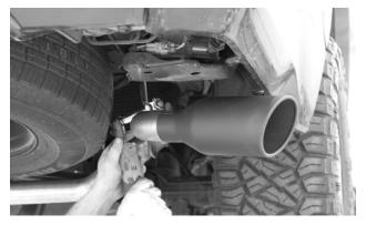
**16.** Install a tip (10) on each exit pipe. Align each tip as desired, and tighten its clamp.
