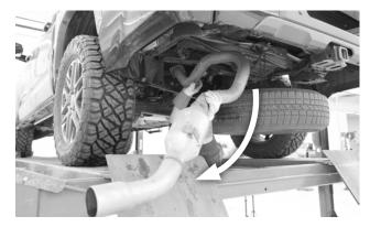
**3.** Lower the spare tire for clearance, and remove the tailpipe from the vehicle.
