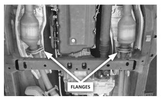
**4.** Remove and retain 4 screws and springs at the 2 catalytic converter flanges.
