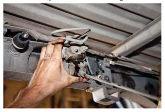
**STEP 4 - REMOVE SPARE TIRE CARRIER** Remove the spare tire carrier.
