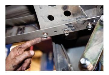
**STEP 5** - **REMOVE SHOCK MOUNTS** Remove upper shock mounts on both sides.
