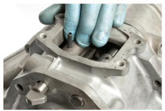
**STEP 47** Place ball in to ball hole on main shaft.
