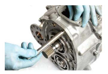
**STEP 29** Remove input gear.
