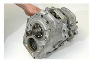
**STEP 30** Remove counter shaft gear.
