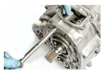
**STEP 46** Apply grease to ball hole on main shaft.
