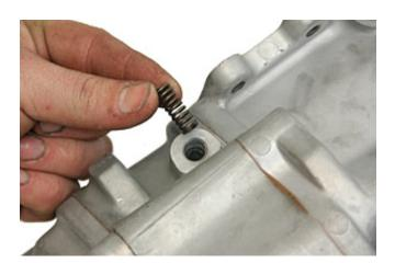
**STEP 72** Install 4wd shift light switch into housing #1.
