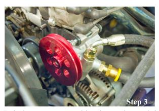
Bolt the new pump and bracket to the stock idler pulley using the provided hardware. Install the new fan belt provided with the kit.
