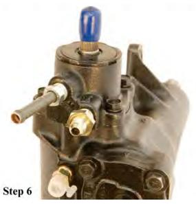
Install the provided high pressure adapter fitting into the steering box. The stock low pressure fitting will be reused. Now connect the lines as shown in the flow photo. The black line is the high pressure hose. The blue lines are low pressure return lines. *Note* that the larger tube is used to connect the reservoir to the pump inlet. **Do not** use smaller 3/8" hose in this location as it will interfere with sufficient fluid
