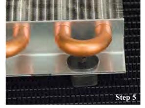
The cooler needs to be mounted which can be done in two different ways. The cooler can be mounted with the ties going through the radiator using the parts provided in the kit or create a frame in front of the radiator, then bolt the cooler to the frame work using the tabs mounted on the back of the cooler.
