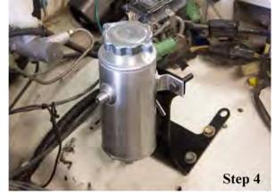
Install the reservoir and bracket in the stock location. The reservoir bracket should line-up with at least 3 holes on the inner fender well on the 1984-1995 4cyl Pick up and 4Runner 4wd applications.
