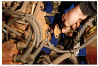
**STEP 7** - REMOVE INTERMEDIATE HEADER TUBE
