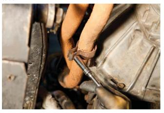
**STEP 3** - REMOVE HEAT SHIELD
