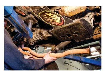
**STEP 11 - REMOVE HEAT SHIELD**
