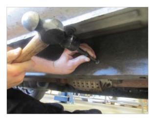
**STEP 7** Use ½" drill bit to drill final holes in frame
