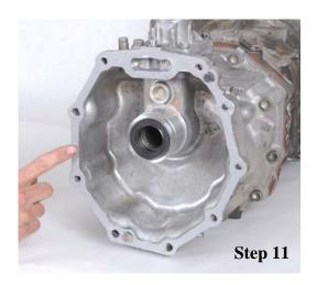
Step 11: Apply silicone to rear face of transmission
