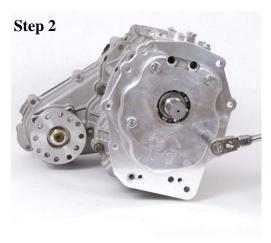
Install adapter plate on face of transfer case, using 4 M10-1.25x35 bolts (provided). We recommend applying blue LocTite® to threads before installation. Torque four plate bolts to 30 ft. lbs.
