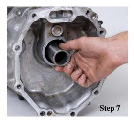
Slide coupler into place on the back of the transmission.
