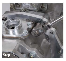
The second allen head bolt should be installed in position shown on the upper right (passenger) side.
