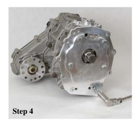
Install M-10-1.25x 35 bolt using blue LocTite $\mbox{\ensuremath{\mathbb{B}}}$  torque to 30 ft. lbs.
