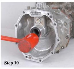
Install Seal Adapter into rear of transmission. Gently seat seal adapter into place using rubber mallet
