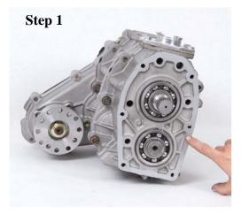
Apply silicone to face of single or dual transfer case assembly.
