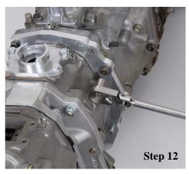
Using 6 of the 9 stock bolts, 1 allen head bolt and 2 M10-1.25x35 bolts, attach transfer case to transmission. Use blue LocTite® on all bolts. Tighten bolts to 30 ft. lbs.
