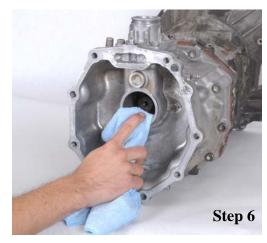
Using degreaser, clean the rear transmission seal surface.
