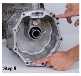
Ensure two dowels are in place in the transmission. If dowels are in the transfer case move them to the transmission.
