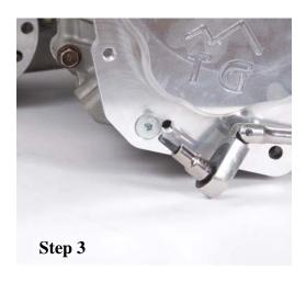
Install M-10-1.25x30 allen head bolt using blue Loc-Tite® torque to 30 ft. lbs.
