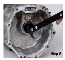
Remove rear transmission seal using a seal remover or claw hammer.
