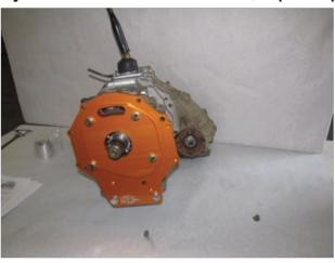
**STEP 4**Install provided coupler to the transmission.
