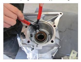
**STEP 9**Remove the rear support bearing.
