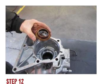
Re-attach the rear transmission housing with 7 bolts and install sleeve.
