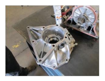
**STEP 8**Remove the rear tranmission seal.
