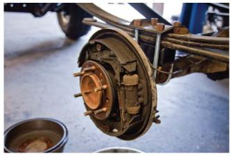
**STEP 4 - REMOVE BEARING POCKET NUTS** Remove the 4 nuts holding bearing pocket in place on each side.
