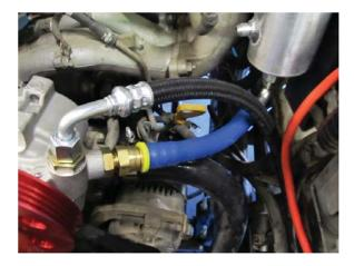
**STEP 19**Route the hoses through a hole in the radiator support.
