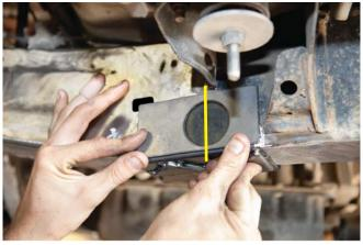
**STEP 53** Mark the frame through the holes in the bottom of the jig.
