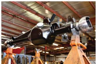
**STEP 123** Rock Assault<sup>™</sup> axle housing with vented rotor and V6 caliper installed.
