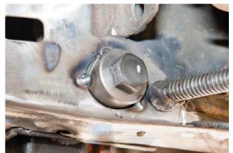
Once the shackle mount is tacked into the frame, clamp the support plate to the frame and tack it into place.
