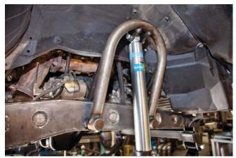
**STEP 95** Install shock hoop support tubes.
