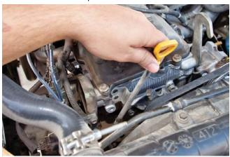
**STEP 23** Place freeze plug in stock dipstick hole.
