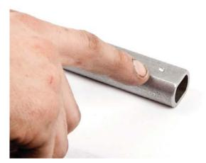
**STEP 113** Loosen the set screw to allow for adjustment.
