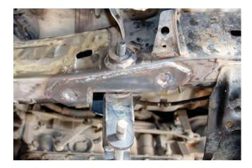
STEP 76 Tack weld the spring hanger into place, centering it upon the mount.
