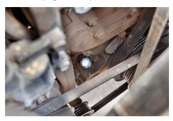
**STEP 22** Apply Ultra Grey to bottom of freeze plug.
