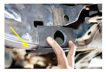
**STEP 54** Outline the jig on the inside of the frame as shown.
