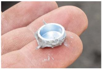
**STEP 24** Lightly tap freeze plug to secure it into place.
