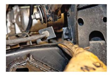
**STEP 17** Grind the frame clean.
