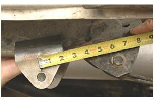
For 1989-1995 Pickups only. The 1989-1995 Pickups used longer spring than the earlier trucks. Follow the spring hanger mounting instructions above but change the dimensions from 6" to 5" so that the hanger is mounted 5" forward of the stock mount.
