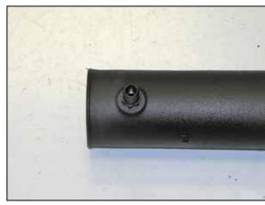
19. Install the provided NPT vent fitting into the  $K\&N^{\odot}$  intake tube as shown.
