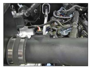
22. Reconnect the mass air sensor electrical connection.
