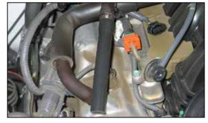
23. Install the crank case vent hose assembly into the factory crank case vent hose as shown.
