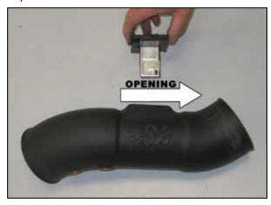
20. Install the mass air sensor assembly into the  $K\&N^{\ensuremath{\circledast}}$  intake tube so that the opening in the sensor faces the filter end of the tube as shown.
