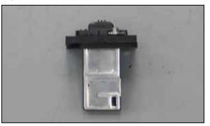
19. Install the mass air sensor through the K&N^ $\ensuremath{\mathbb{R}}$
