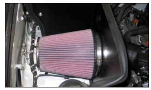
26. Install the K&N<sup>®</sup> air filter and secure with the provided hose clamp.
