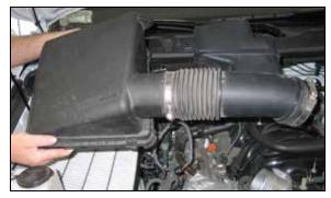
6. Release the four retaining clips securing the upper air box and then remove the upper air box and intake tube assembly from the vehicle.
