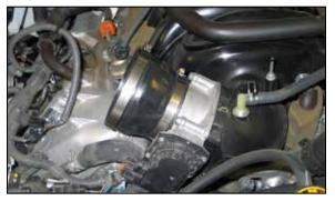
15. Install the silicone hose (08497) onto the throttle body and secure with the provided hose clamp.
