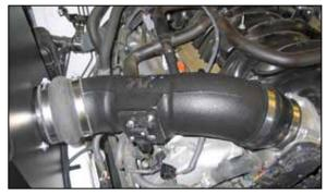
24. Insert the K&N<sup>®</sup> intake tube into the hump hose attached to the heat shield and then into the step hose attached to the throttle body. Secure with the provided hose clamps.
