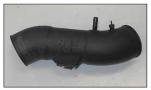
21. Install the provided NPT vent fittings into the  $K\&N^{\circ}$  intake tube as shown.
