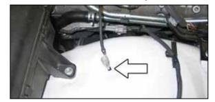
2. Disconnect the mass air sensor electrical connection and unhook the wiring harness from the air box.
