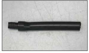
22. Install the hose mender into the provided crank case vent hose as shown.
