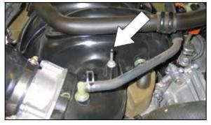
28. Remove the front engine cover mounting stud from the intake manifold.
