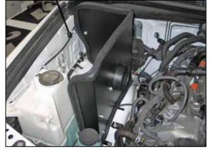
14. Set the heat shield into the engine compartment and secure the factory nuts and with the provided hardware.
