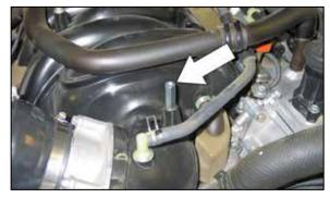
30. Install the provided nut extension onto the stud as shown.
