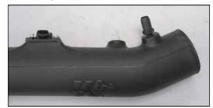
26. Install the 5/8 vent fitting into the  $K\&N^{\otimes}$  intake tube as shown.
