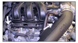
30. Connect the provided fuel pressure vent line to the fuel pressure regulator and then connect the open end to the 3/16 vent fitting in the K&N<sup>®</sup> intake tube.
