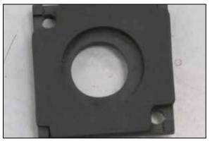
22. Install the provided gasket onto the K&N $^{\mbox{\tiny \$}}$  mass air sensor adapter as shown.
