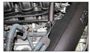
35. Reconnect the mass air sensor electrical connection.
