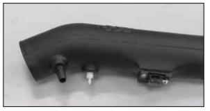
27. Install the 3/16 vent fitting into the K&N® intake
