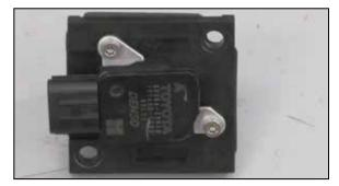
24. Install the mass air sensor into the K&N<sup>®</sup> mass air sensor adapter and secure with the provided hardware.
