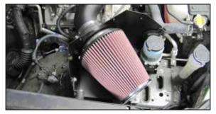
31. Install the K&N<sup>®</sup> air filter onto the filter adapter and secure with the provided hose clamp.
