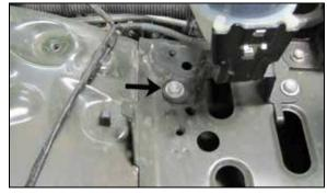
10. Remove the rear P/S reservoir mounting bolt shown.
