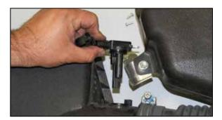
23. Remove the screws which secure the mass air sensor to the factory air box and then remove the mass air sensor from the air box.
