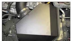
33. Install the heat shield cover onto the heat shield and secure with the provided hardware.NOTE: Use of the heat shield cover is not
