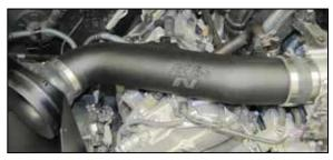
28. Install the K&N<sup>®</sup> intake tube into hump hose at the filter adapter and then into the silicone hose at the throttle body, align the tube for proper fit and then tighten the hose clamps.
