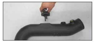
25. Install the mass air sensor assembly into the K&N<sup>®</sup> intake tube and secure with the provided hardware.
